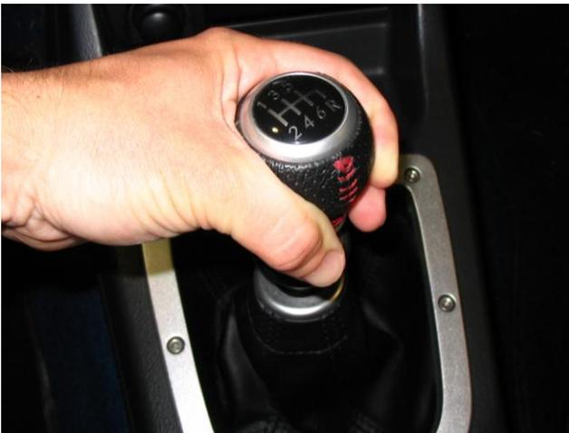
1. Ensure that your parking brake is engaged inside the car. Unscrew stock shift knob by rotating counter clockwise.
