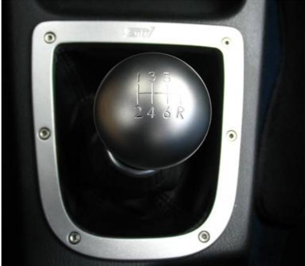
13. Re-install the shift knob and tighten down by hand. If the insert was adjusted correctly the engraving will line up properly. If the logo does not quite line up properly, remove the shift knob and repeat steps 8 to 12 to adjust the insert and jam nut to line it up. Only minor adjustments should be required at this point.
