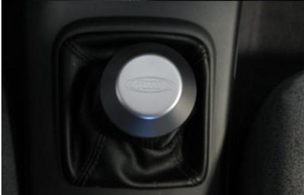
**PLEASE NOTE:** if you re-adjust the knob, loosen the jam nut **FIRST** by holding the aluminum insert with a 15mm wrench and rotating the jam nut **CLOCKWISE**. Do not loosen the insert first, simply hold it with the wrench and loosen the jam nut to maintain approximately the correct orientation of the insert.
