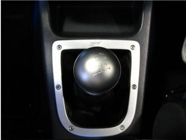
8. Pictured to the left is the point where the insert encounters the top of the inside of the shift knob (or the height adjuster screw) and it stops turning. Notice how the TWM logo (or shift pattern) on the shift knob is not aligned correctly. Make a note of how much the shift knob needs to be backed off to align the engraving (or logo), in this case it needs to be backed off slightly less than  $\frac{3}{4}$  turns.
