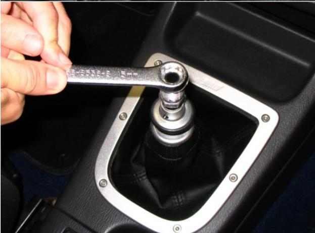
10. Pictured to the left is the insert in it's final resting position once it has been backed off counter clockwise to ensure proper engraving alignment. Continue to hold the insert in this position.
