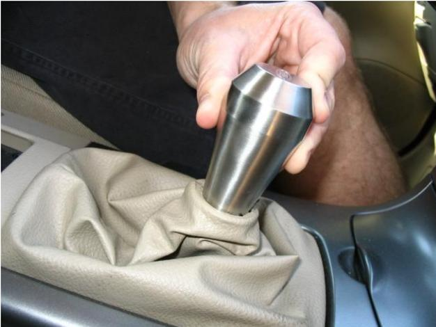
3. Test the height of the shift knob by sliding it over the shifter shaft. Adjust the height with the special tool if necessary. You will need to leave approximately 1" inch of free threads at the bottom of the shift knob to cover the aluminum insert and low profile jam nut when the shift knob is threaded on to the insert.
