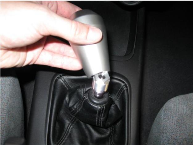
7. Thread the shift knob on to the aluminum insert until you experience resistance, this is the point where the aluminum insert encounters the height adjuster set screw or the end of the inside threads if you did not use the height adjuster screw. If you have a shift knob with no logo/engraving, you are done! If you want to re-adjust the height of the shift knob, repeat steps 2 and 3.
