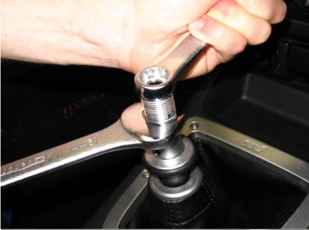
12. Still holding the insert in position with the 15mm wrench, use a 9/16" open ended wrench to tighten the jam nut up against the bottom of the insert. Do not tighten the insert down as this will change the logo orientation. Simply hold it in position while tightening the jam nut from below. The jam nut is tightened against the insert by rotating counter clockwise.
