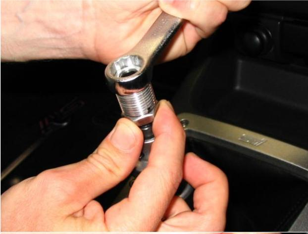
11. While still holding the insert in place, thread the jam nut up the shaft (counter clockwise) until it touches the bottom of the aluminum insert.
