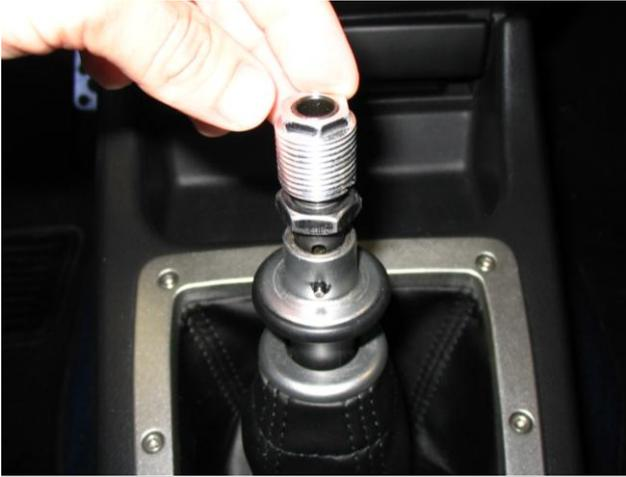
5. Thread the supplied aluminum insert on to the shifter shaft by hand with the hex end facing up.
