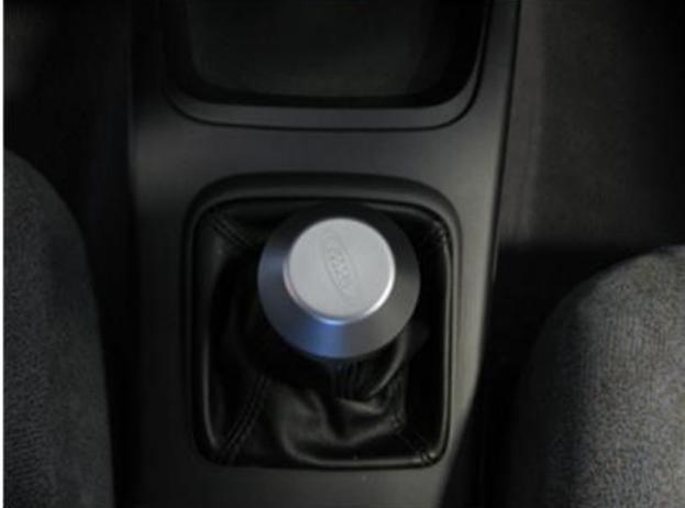
Please note that it is impossible to thread the insert deeper to align the engraving, the insert **MUST BE BACKED OFF COUNTER CLOCKWISE**.
