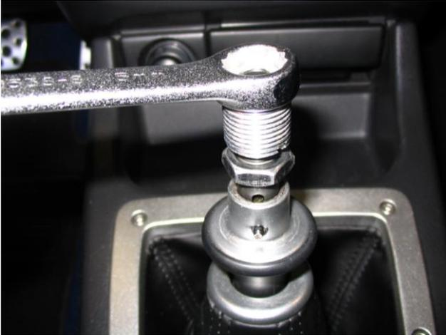
6. Now lightly tighten the aluminum insert on to the shifter shaft. A 15mm wrench can be used to tighten the insert. The insert should only be snug on the shaft, do not over tighten.
