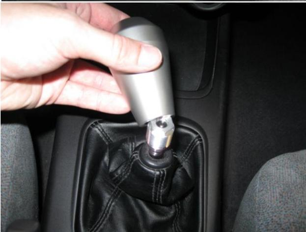
9. Unscrew the shift knob leaving the aluminum insert in place on the shaft. This will allow access to adjust the jam nut and insert to set proper engraving or logo alignment.
