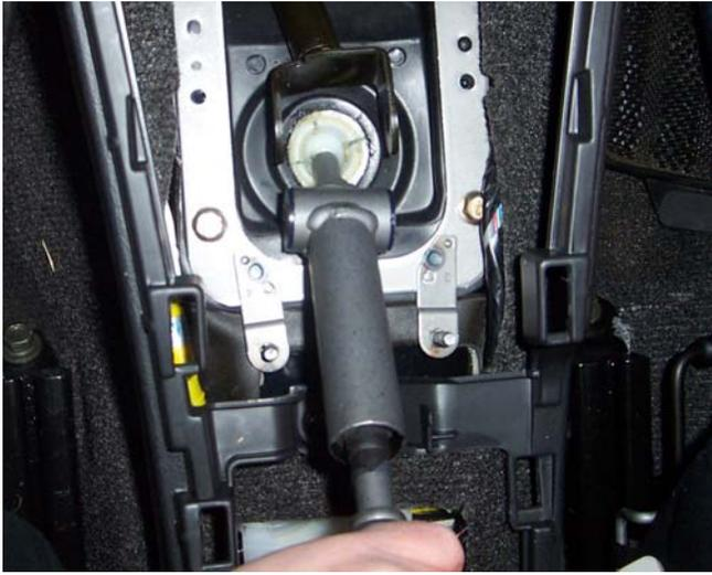
6. Remove the stock shifter by prying back and downward. The white plastic ball will pop out of the cup at its base. Push out the steel cross sleeve in the stock shifter with your finger and clean it with a shop towel, re-greasing it afterward. Remove the rubber bushings on either side of the shifter and clean them with a shop towel. These will be re-used in the installation of the TWM shifter.
