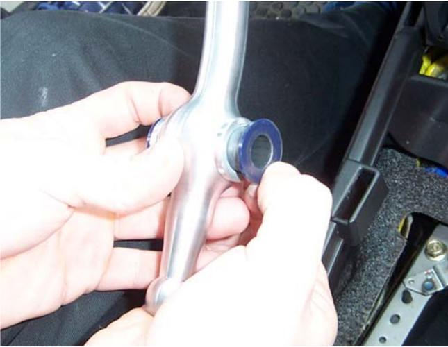
7. Install the rubber bushings you removed from the stock shifter in the previous step into the TWM shifter.
