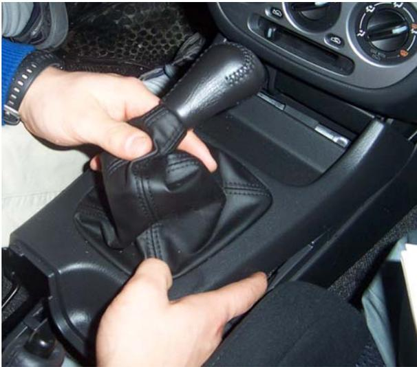
4. Unscrew the shift knob and separate it from the shift boot. Lift up on the front portion of the center console and it will pop out.
