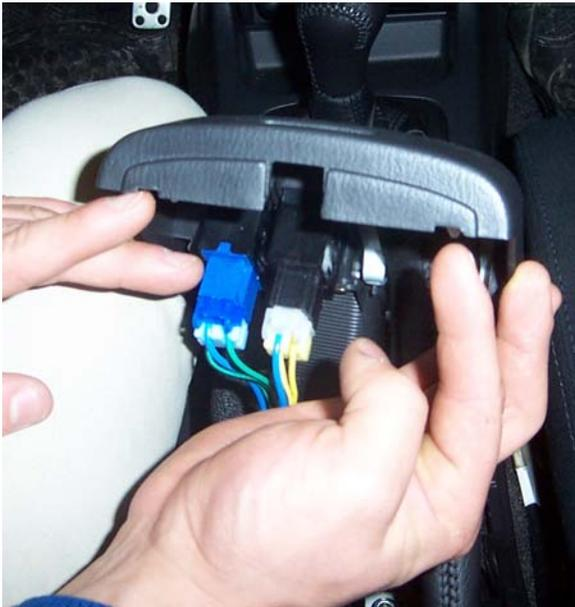
2. Disconnect both plastic connectors beneath the rear part of the center console. Note their locations for re-installation.
