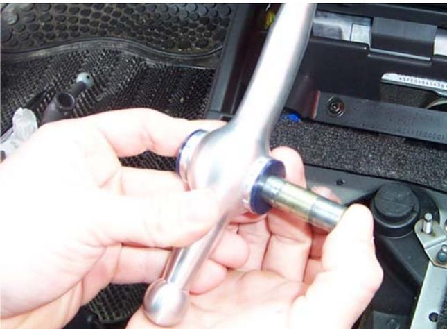
8. Insert the steel cross sleeve that you removed from the stock shifter in step 6 into the TWM shifter.
