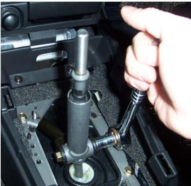
5. Unscrew the nut securing the shifter to the shift rod. Remove the bolt that passes through the shifter and shift rod, place the nut and bolt in a clean area, they will be used for re-installation.
