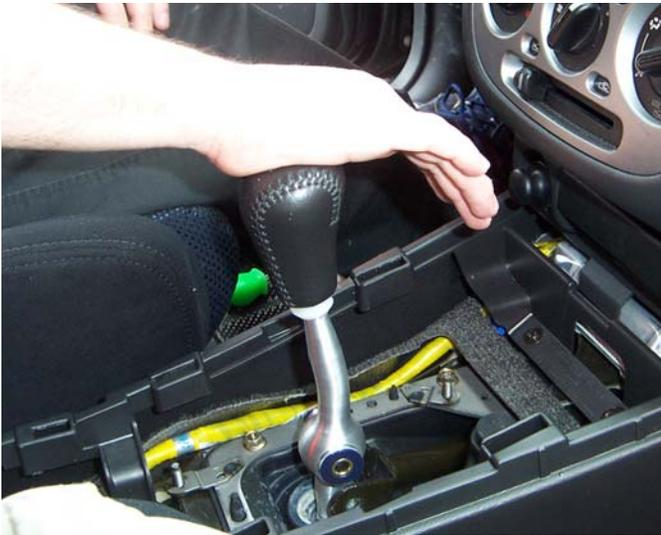
10. Screw the shift knob on to the TWM shifter. Use the palm of your hand to force the shifter to pop into plastic pivot cup at the base. This may require a strong impact using the palm of your hand to pop it in. Remove the shift knob once the TWM shifter is popped in to the base cup.
