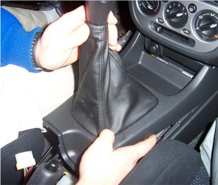
12. Re-assemble the console, first installing the front half. Replace the shift knob in to the boot and thread it on to the TWM shifter. Re-connect all plastic connectors in the same manner as they were to the rear portion of the console. Snap the rear portion of the console back into place and you're ready to drive!
