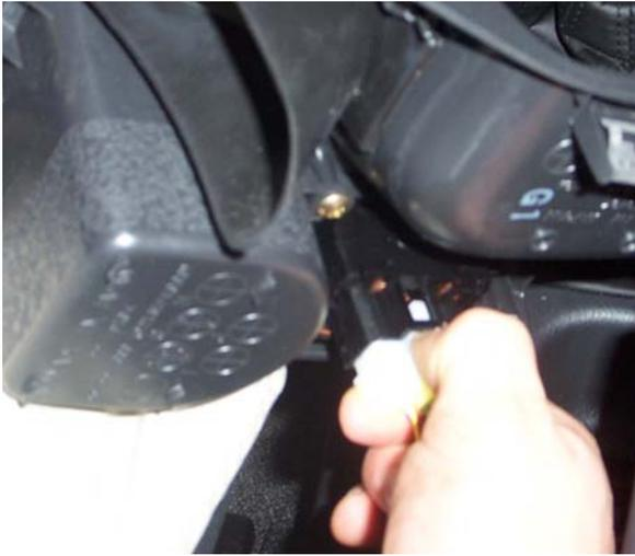
3. Disconnect the larger plastic connector at the front of the rear part of the center console. Remove the rear part of the center console and place it in a safe area.
