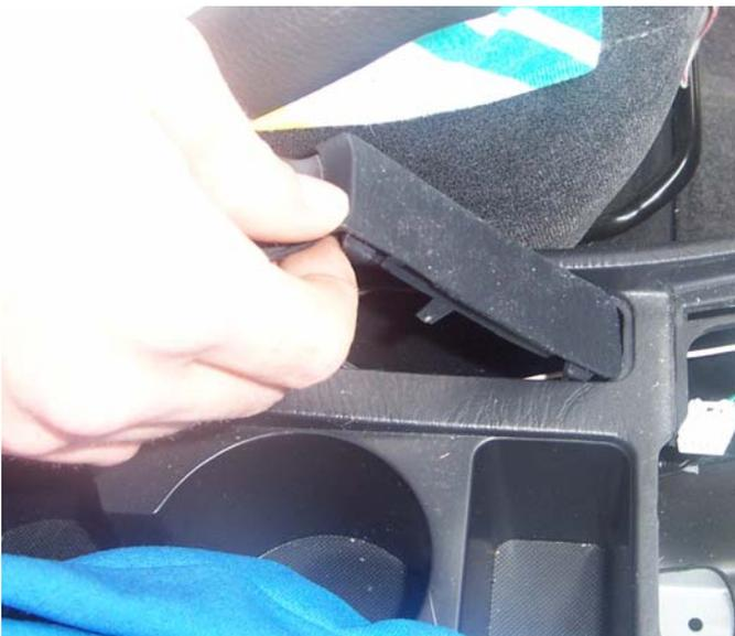
5. Remove the plastic cover in front of the handbrake.
