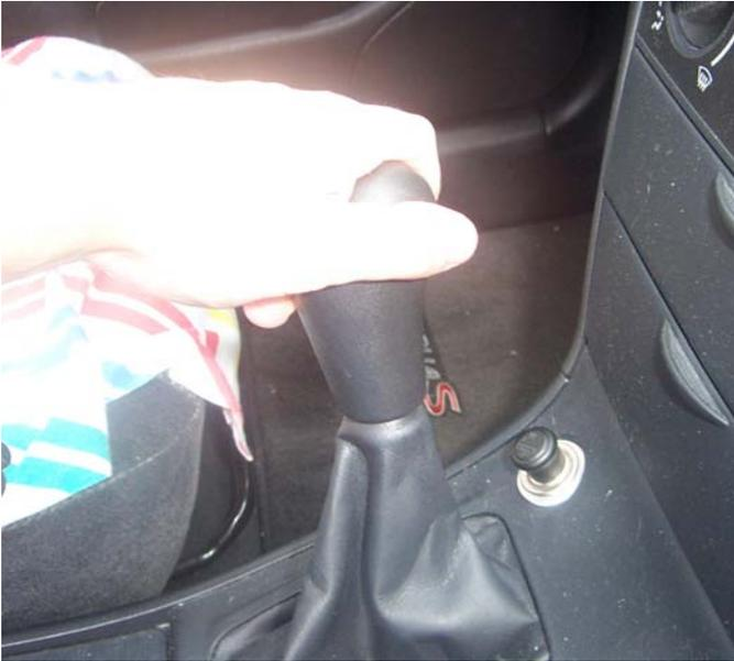
1. Unscrew the shift knob and remove the boot.
