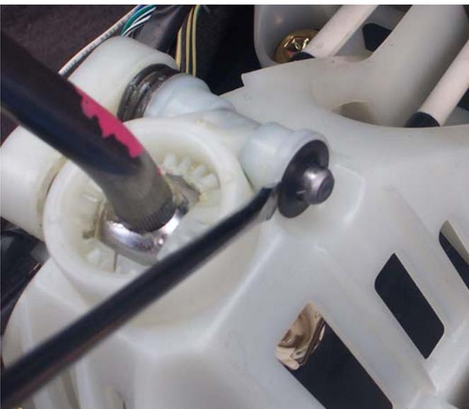
11. Insert a flat head screw driver behind the clip on the right front side of the assembly and pry the clip off. The clip may be broken in the process but a new one is included with the TWM shifter.
