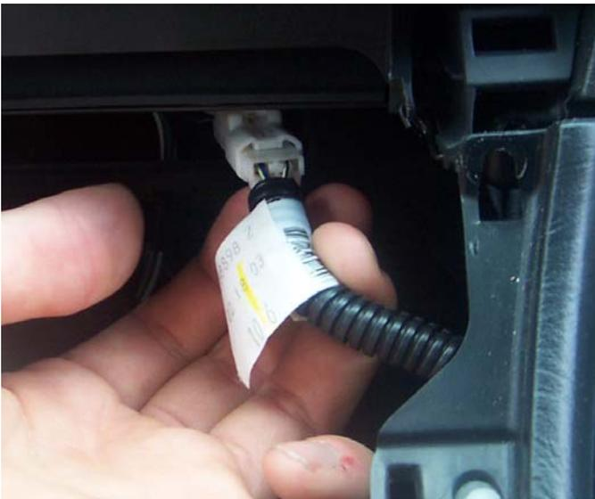
7. Unclip the plastic connector at the front of the console.
