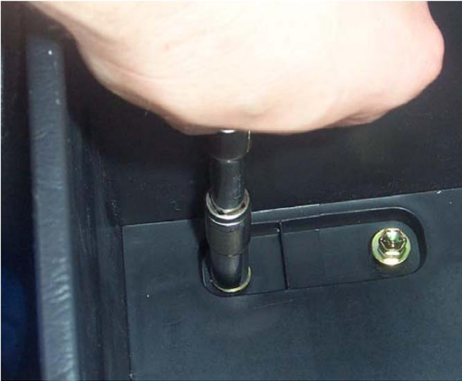
6. Remove the rubber mat, and the two bolts in the storage compartment of the center console.
