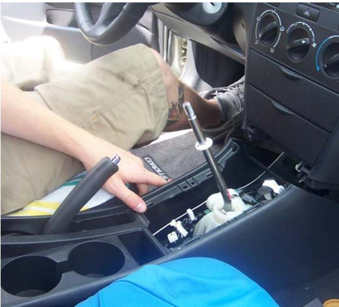
8. Carefully lift and remove the console from the car to allow access to the shift assembly.
