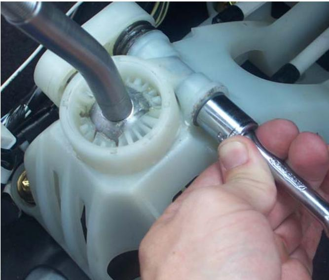
16. Drive the clip on with a 14mm socket to secure it properly against the plastic assembly. Be sure the shaft is pushed all the way into the assembly and the clip is on all the way so there is no free play.
