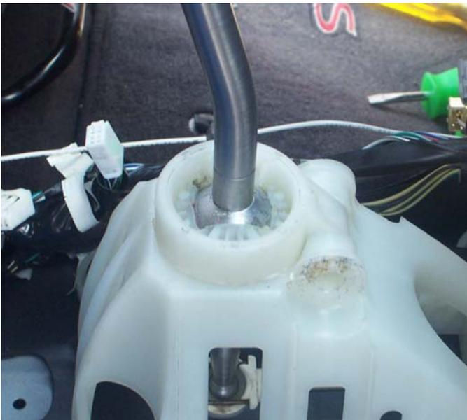
14. Lightly grease the large pivot ball and the small side pivot ball on the TWM shifter. Install the TWM shifter in place of the stock one and replace the plastic cap by pressing it on firmly until it snaps into place.
