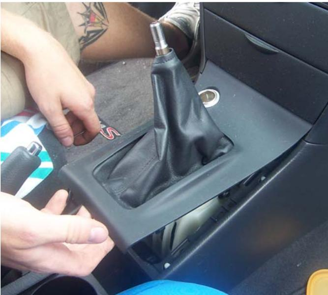
2. Remove cover which houses the lighter assembly. Lift it gently and it pops out.
