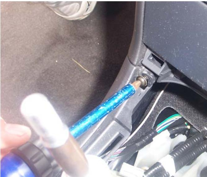
4. Remove the 2 screws at the front of the console.
