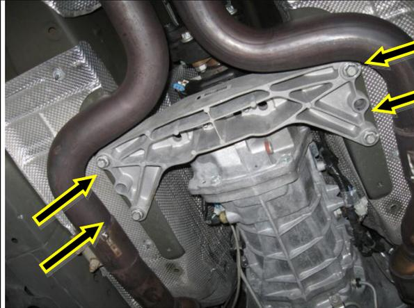
6. Next, the transmission support needs to be taken off, with the same 15mm socket, remove the (4) screws holding the support to the body
