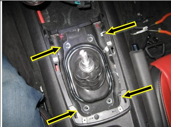
4. Loosen, but not remove, the (4) screws holding the shifter assembly to the body using a 10mm socket
