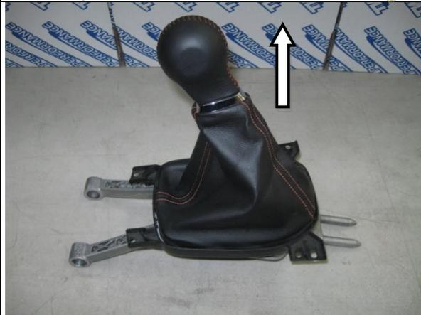
3. Remove the shift knob by pulling upwards with some force
