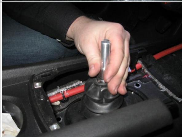
12. Then insert the shifter shaft, having a friend in the car to guide the shaft through the upper dust boot is very helpful
